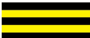
Continuous taxiway edge markings are used to delineate the taxiway edge from the shoulder or some other contiguous paved surface not intended for use by aircraft. The markings consist of a continuous double yellow line, with each line being at least six inches in width and spaced six inches apart.
