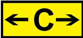
These signs indicate directions of other taxiways leading out of an intersection. The signs have black inscriptions on a yellow background and always contain arrows. The arrows are oriented to approximate the direction of the turn. The signs are lighted at night or during limited visibility operations.
