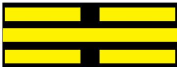
An enhanced taxiway centerline marking consists of a parallel line of yellow dashes on either side of the existing taxiway centerline. Taxiway centerline markings are enhanced for 150 feet prior to a runway holding position marking. The purpose of these markings are to identify to a pilot or vehicle operator that they are approaching the runway holding position.
