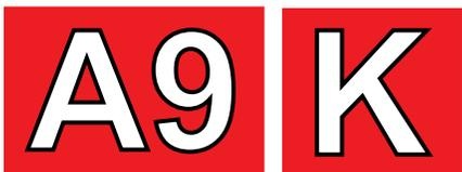
LAHSO is used by ATCT to land aircraft on a runway while guaranteeing that the aircraft will hold short of a specific point. At MSP LAHSO is used on Runway 30L to hold short of A9 and on runway 22 to hold short of K. There are Holding Position Signs, Holding Position Markings and in-pavement lighting for each of the LAHSO points.
