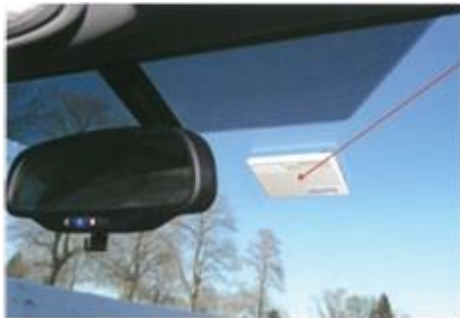
Proper mounting of Transponder
