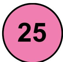
These markings consist of a number painted inside a seven foot diameter pink circle. These markings are installed when points are necessary to identify the location of taxiing aircraft during low visibility operations. Low visibility operations are those that occur when the runway visual range (RVR) is below 1200 feet.
