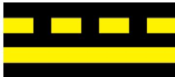
Non-movement area boundary markings are used when there is a need to delineate the movement area from the non-movement area. The markings consist of two yellow lines (one solid and one dashed). The solid line is located on the non-movement area side while the dashed yellow line is located on the movement area side.
