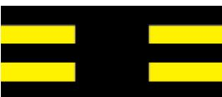
Dashed taxiway edge markings are used when there is an operational need to define the edge of a taxiway or taxilane on a paved surface where the pavement next to the edge is intended for use by aircraft. The markings consist of a broken double yellow line with each line being at least six inches in width and spaced six inches apart. The lines are 15 feet in length with gaps of 25 feet.
