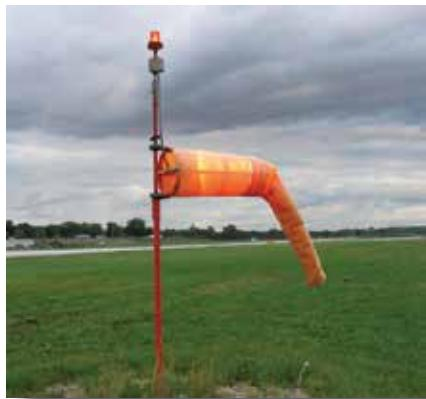
These are located along the runways and are lighted during periods of darkness or reduced visibility. The wind socks are made of flexible fabric and move freely when subjected to air movement. The wind socks indicate the wind direction and wind force by noting which way the sock is pointing and whether the sock hangs limply or is extended. The sock points to the direction
