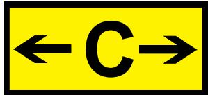
These signs indicate directions of other taxiways leading out of an intersection. The signs have black inscriptions on a yellow background and always contain arrows. The arrows are oriented to approximate the direction of the turn. The signs are lighted at night or during limited visibility operations.
